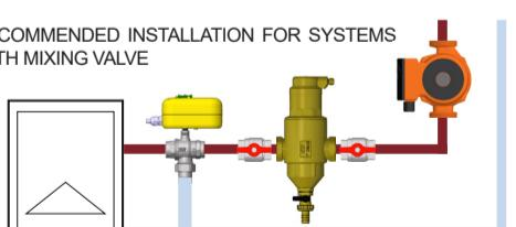
**Note!** To operate efficiently, the deaerator should always be installed in a horizontal pipe run, with the body upright.
